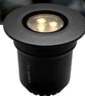
Nomia [207U] Aluminium - noir LED 3W 3.000K - 313lm 86 x 90 mm (HxØ) Trou de forage 70 mm
